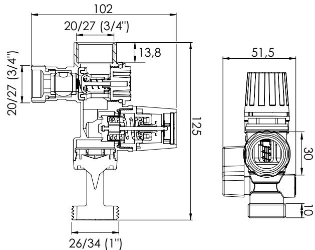
**SIÈGE EN TÉFLON ADAPTÉ AUX EAUX CALCAIRES**
