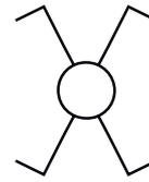
Intermediate switch circuit
