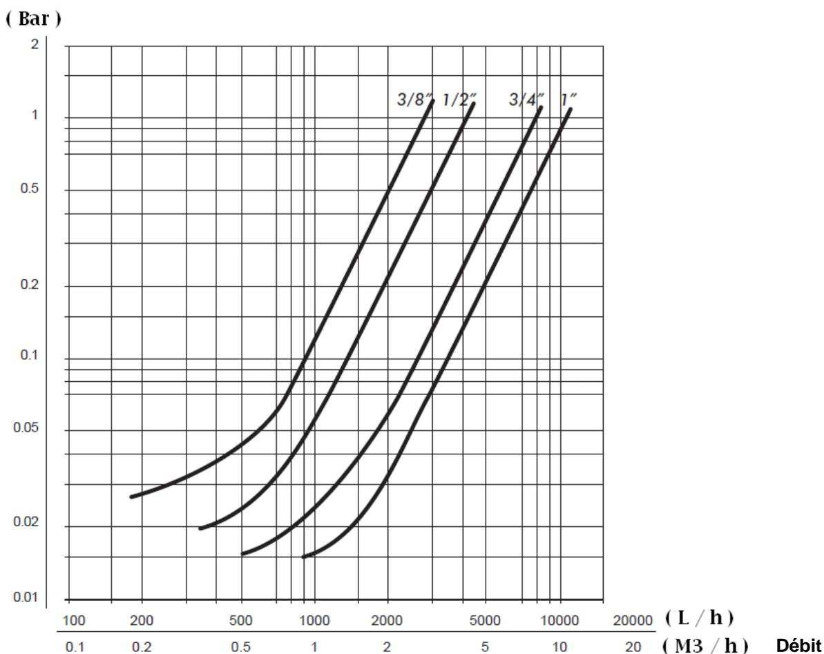
**CLAPET DE NON RETOUR A DOUBLE GUIDAGE LAITON 4MS MALE-FEMELLE ACS**
