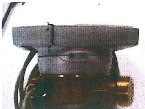
Figure 4 –Heat meter sealing of the calculator after positive initial verification
